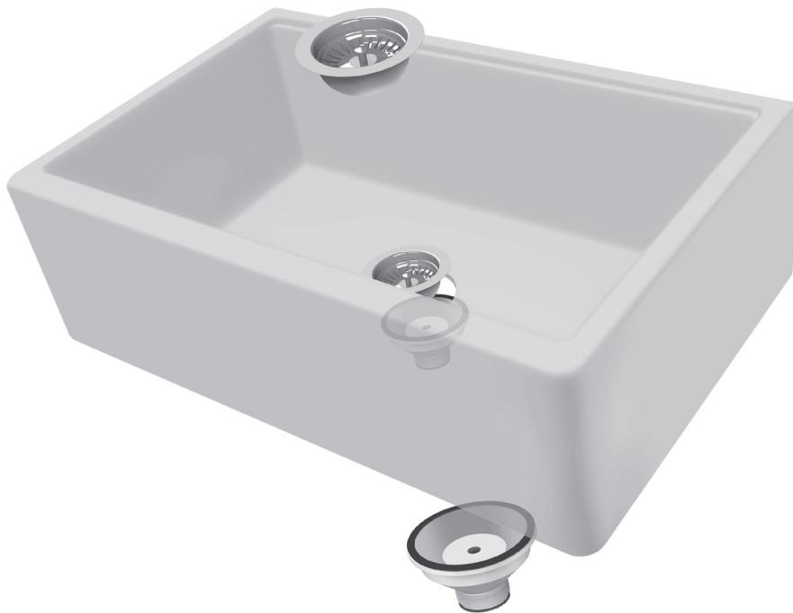
2) Fasten the strainer to the drain using the provided screw. Do not overtighten.
